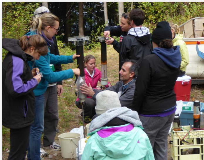
Sectioning the Sediment Cores
