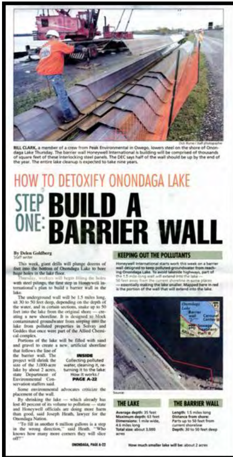
The barrier wall prevents contaminated groundwater from entering Onondaga Lake.
