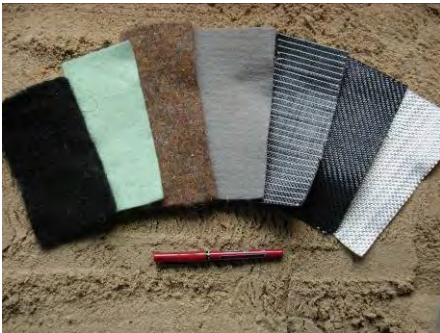
Geotextiles are permeable fabrics that have the ability to separate, filter, reinforce, protect, or drain when used in association with soils.
