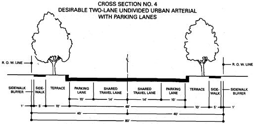
NOTE: A 4-INCH WIDE SOLID WHITE STRIPE OR MARKED PARKING STALLS SHOULD BE USED TO DISTINGUISH THE TRAVEL LANE FROM THE PARKING LANE.
