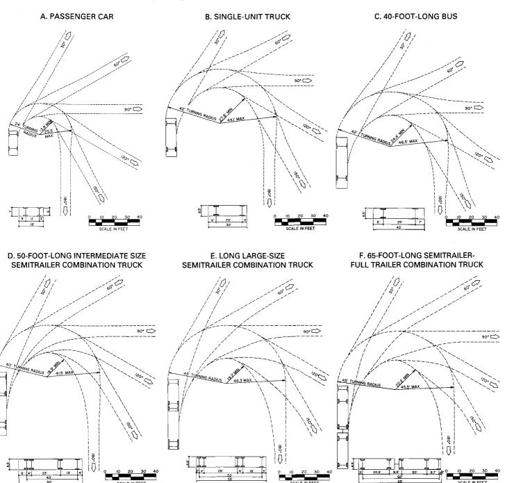
NOTE: The turning templates show the turning paths of the AASHTO design vehicles. The paths shown are for the left front overhang and the outside rear wheel. The left front wheel follows the circular curve, however, its path is not shown.
