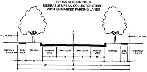
NOTE: IF THE RIGHT-OF-WAY WIDTH IS LIMITED, THEN THE TERRACE CAN BE REDUCED TO 7 FEET WIDE.
