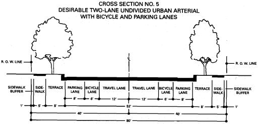
NOTE: A 6-INCH WIDE SOLID WHITE STRIPE SHOULD BE USED TO DISTINGUISH THE TRAVEL LANE FROM THE BICYCLE LANE. A 4-INCH WIDE SOLID WHITE STRIPE OR MARKED PARKING STALLS SHOULD BE USED TO DISTINGUISH THE BICYCLE LANE FROM THE PARKING LANE.
