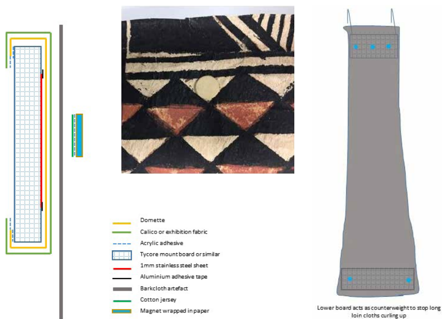
Figure 21.4. Diagrammatic representations of the magnet mounting system used to hang the barkcloth.
