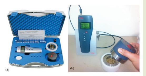
Figure 1. The Portable water activity meter (a) packed for transport and (b) in use at the BC Tree Seed Centre.
