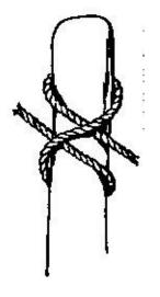
Used to fasten one pole to another in fitting up scaffolding; this knot holds snugly; is not liable to slip laterally. Hold the standing part in left hand, then pass the rope around the pole; cross the standing part, making a second turn around the pole, and pass the end under the last turn.
