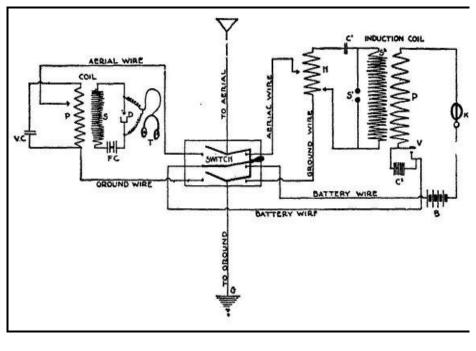
The first thing to do is to build an aerial. First find out how long your location will allow you to build it, and how high. It ought to be at least 50 to 60 feet high and about 70 to 100 feet long. The main point in building an aerial is to have it {211} well insulated from the ground, and all connections in wire perfectly solid. It is advisable to solder every connection and to make your aerial strong as it has a great deal to do with the working qualities of the station.
