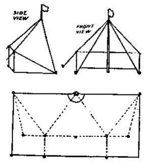
Fig. 8. So-called canoe tent. Requires three guy lines, and can be supported by a rope instead of a pole
