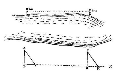
To measure the space between two distant objects, D and E. Line A B on one, then move this right-angled triangle until F G is lined on the other, with B G in line with G H. B G
