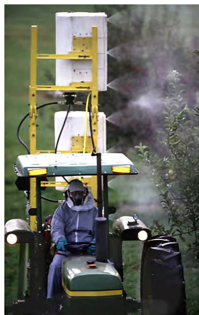
Air-curtain orchard sprayer in an apple orchard. Photo by Keith Weller, USDA Agricultural Research Service.
