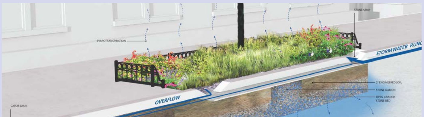
Right-of-way bioswales in NYC use the street slope, curb, and channel to intercept stormwater runoff before entering catch basins (photo from NYC DEP Green Infrastructure website)
