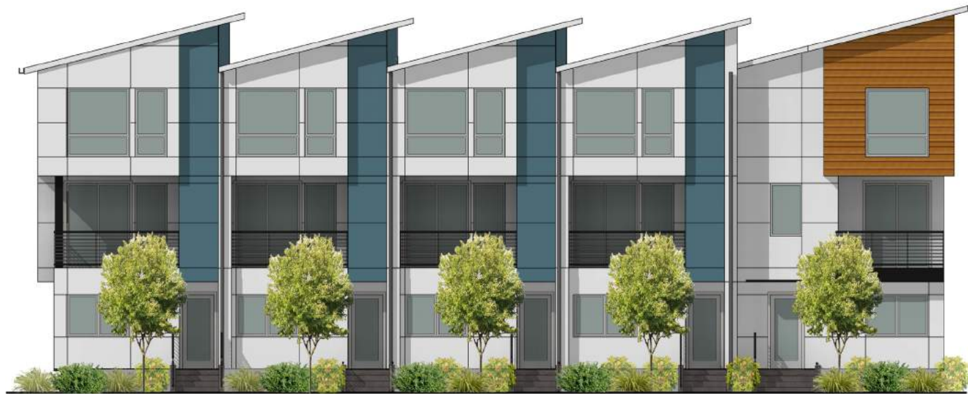
FRONT ELEVATION - SHED ROOF (BUILDING F SHOWN) USED ON BUILDINGS C, D, E, F, G, H
