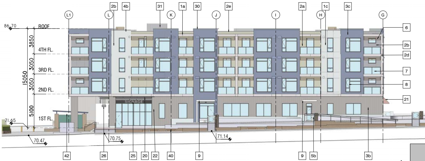
1 NORTH ELEVATION BUILDING B SCALE 1:96
