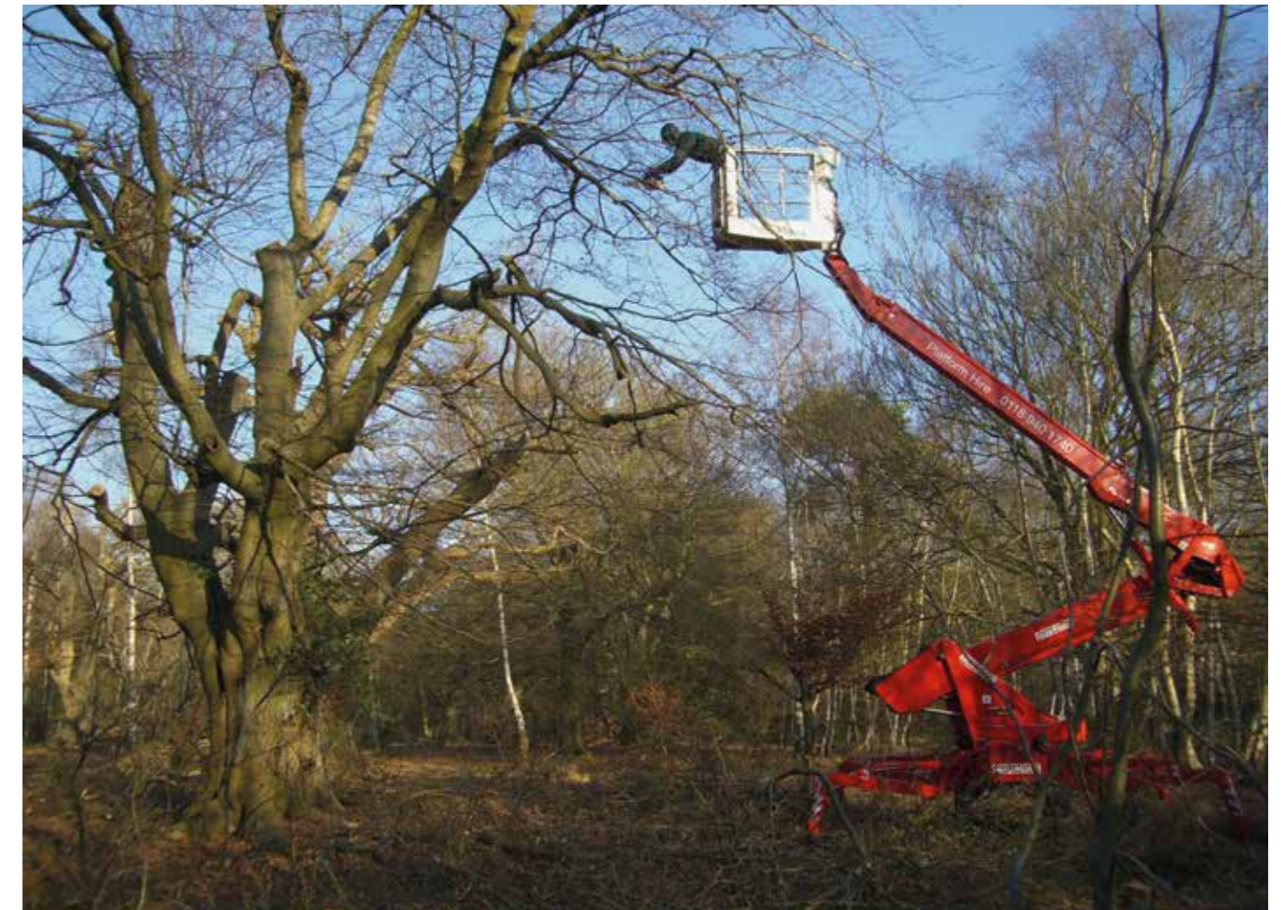
▲ Pruning of ancient trees is a last resort. At Burnham Beeches (U.K.) an access platform is used to reduce the height and weight of trees vulnerable to falling apart. (© City of London).
