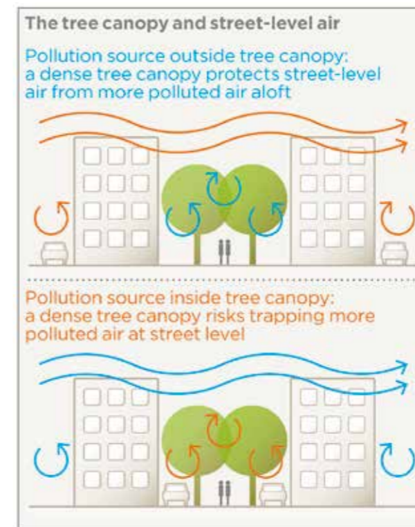
▲ Figure 3. The effect of a dense avenue of trees in an urban canyon depends on whether the air at street level is cleaner or more polluted than the air above it. By reducing mixing between the two, a dense canopy on a quiet street protects relatively clean air at street level from the import of polluted air from above (top panel). On a busy street, however, a dense canopy risks trapping pollution at street level (bottom panel). 13 (© Trees and Design Action Group Trust).
